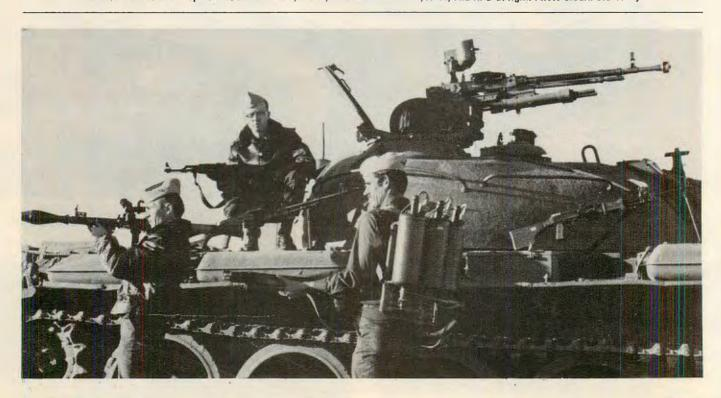
The T-54, 55, and 62 all have four-man crews. The T-54 and 55 mount a 100mm rifled main gun, 7.62 MG, and a 12.7mm (.50 caliber) DShK 1938/46 heavy MG for anti-aircraft use. Some of these tanks have chemical, biological, radioactive (CBR) equipment, which may be manually operated or activated by an atomic weapon flash.
